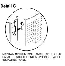
Figure 6. Removing and Installing Panels
